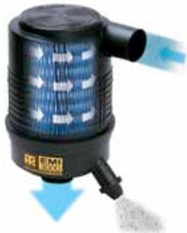
EMI-3000 air filters offer the greatest efficiency in air filtration for Thermo King equipment via the two-stage cyclonic action process. 75% of the particles are removed from the filter out the evacuation valve before they even reach the filter media. This allows only the Thermo King filter to reach maximum efficiency of 99.97%.
